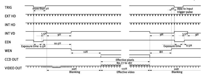
Fig. 13. Vertical timing for Edge pre-select 1/2 partial scanning
